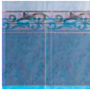
Printing flaws due to irregular belt feed
