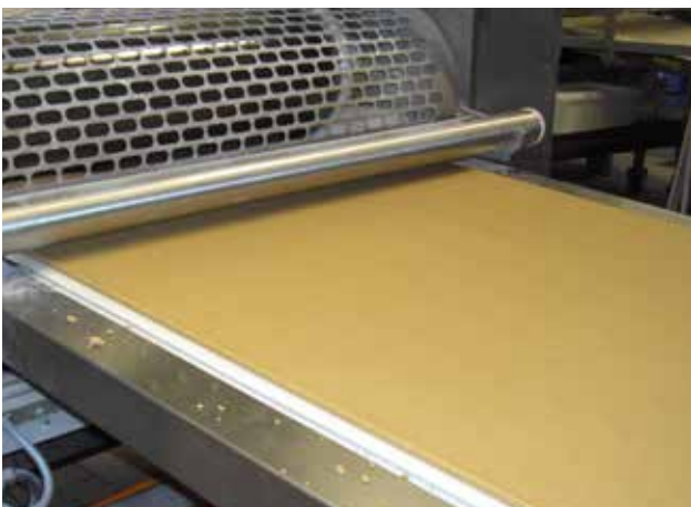
Gauge rolls for dough sheets production
