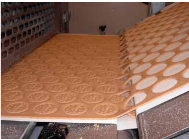
Rotary cutter and scrap return belt
