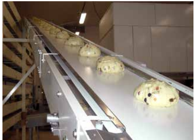
Inclined conveying towards multistory open air proofer
