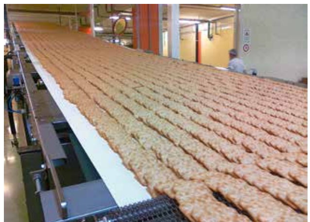
Crackers cooling conveyor
