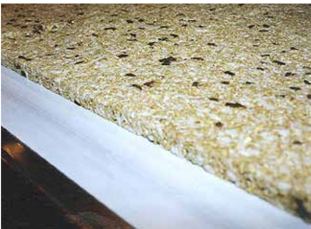
Muesli conveying on a dehesive belt
