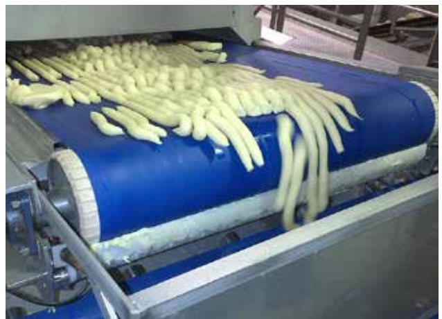
Fries conveying after frying
