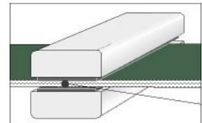
2. Allow the cooling cycle to be completed before removing the belt from the press.
