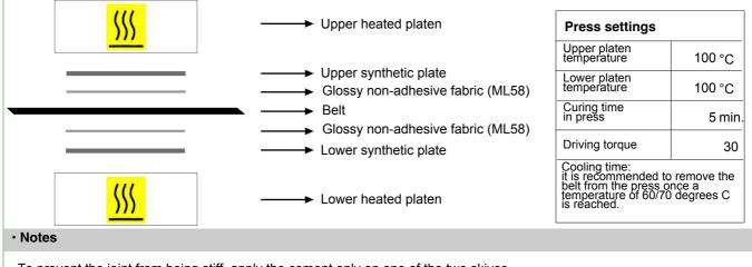
To prevent the joint from being stiff, apply the cement only on one of the two skives.
